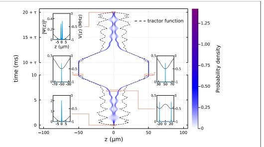
**Figure 4.** Optimized interferometric sequence for scalar TAI. The heatmap shows the probability density  $|\Psi(z,t)|^2$  as the initial wave packet passes through splitting (first 10 ms), free evolution (not to scale), and recombination (last 10 ms). The dashed lines show the tractor functions, i.e., the optimized controls. The insets correspond to selected snapshots of the dynamics showing both the potentials (black lines) and the probability densities (blue lines).
