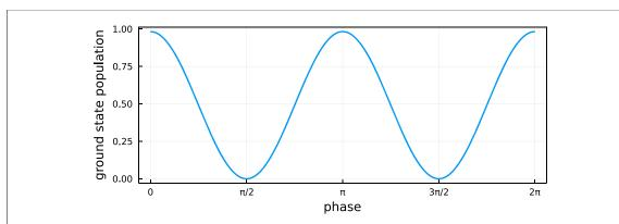
**Figure 5.** Ground state population of the tractor potential at the final time as a function of the accumulated differential phase between the left and the right arm of the TAI. The phase was modeled by introducing an instantaneous phase kick to the wave function in the left potential at  $t = 10 \text{ ms} + \tau/2$ , see figure 4.
