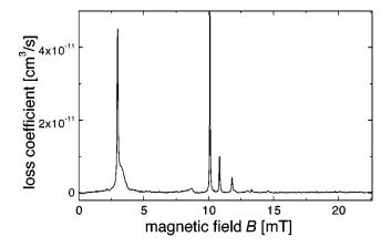
FIG. 4. Binary loss coefficient in a gas of  $|F=3, m_F=-3\rangle$  atoms as a function of external magnetic field. The initial mean atomic density is  $\bar{n}=5 \times 10^{12}$  cm<sup>-3</sup> at a temperature of ~5  $\mu$ K. Populations in the  $|F=3, m_F=-3\rangle$ ,  $|F=3, m_F=-2\rangle$ , and all other states are 95%, ~5%, and <1%, respectively. Magnetic field resolution is 10  $\mu$ T.
