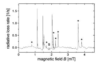
FIG. 6. A detailed radiative loss spectrum. The probe beam at wavelength  $\lambda$ =844 nm has an intensity of 50 W/cm<sup>2</sup>. Here 85% (15%) of the atoms are in the  $|3,3\rangle$  ( $|3,2\rangle$ ) state. The temperature and mean density of the sample are 3.5  $\mu$ K and 1×10<sup>13</sup> cm<sup>-3</sup>, respectively. "S" indicates a shape resonance; the stars indicate Feshbach resonances in the (3,3)+(3,2) channel. Magnetic field resolution near the resonances is 5  $\mu$ T.
