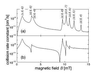
FIG. 11. Collision rate constants in the  $(F=3, m_F=-3)+(F=3, m_F=-3)$  scattering channel at  $E/k_B=1$  nK. Inelastic collision rates (a) and elastic collision rates (b) are calculated with a magnetic field grid size of 10  $\mu$ T for off-resonance regions and 1  $\mu$ T near the resonances. Resonances from the M=-6, s-, d-, and g-wave bound states are included and assigned with quantum number  $(l, f, m_f)$ , where the notation is the same as in Fig. 10.
