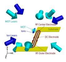
FIG. 1 (color online). Setup for trapping neutral (MOT) and singly charged (surface planar Paul trap) Yb in the same spatial volume. Stray dc field compensation and trapping along  $\hat{z}$  for the Paul trap is provided by dc electrodes. The traps are imaged along both the (1,0,1) and (0,1,1) axes.
