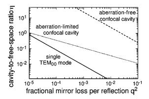
FIG. 3. Cavity-to-free-space scattering ratio  $\eta$  as a function of the fractional mirror loss per reflection for a single TEM<sub>00</sub> mode (solid line), for a confocal resonator without aberration (dashed line), and for a confocal resonator with spherical aberration (dotted line). A resonator of 10 cm length with a mirror radius of curvature of R = 10 cm and a mirror diameter of 2r = 12.7 mm is assumed.
