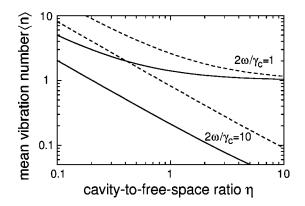
FIG. 4. Mean vibration number  $\langle n \rangle$  for cavity sideband cooling as a function of cavity-to-free-space scattering ratio  $\eta$  along the cavity axis z (solid line) and along the incident beam x (dashed line) for  $2\omega/\gamma_c = 1$  and  $2\omega/\gamma_c = 10$ .  $2\gamma_c$  is the resonator linewidth and  $\omega/2\pi$  the trap vibration frequency.
