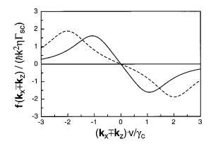
FIG. 2. Cavity Doppler force along a diagonal direction  $\mathbf{k}_x = \mathbf{k}_z$  as a function of Doppler effect  $(\mathbf{k}_x = \mathbf{k}_z) \cdot \mathbf{v} / \gamma_c$  along that direction. The detuning of the incident light relative to the cavity resonance is  $\delta_i = -\gamma_c - 2E_{rec}/\hbar$  (solid line) and  $\delta_i = -2\gamma_c - 2E_{rec}/\hbar$  (dashed line).  $\eta \Gamma_{sc}$  is the on-resonance scattering rate into a single direction of the cavity.
