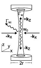
FIG. 1. Setup for 2D or 3D cavity Doppler cooling with a single cavity and multiple incident beams. For 2D cooling a pair of counterpropagating beams along the *x* axis and polarized along *y* is used. 3D cooling is achieved by adding a pair of beams propagating along  $\pm y$  and polarized along *x*.
