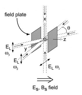
FIG. 1. Proposed experimental configuration. Three standing waves form an optical lattice. They have different frequencies and polarizations that are linear and perpendicular to the quantization axis defined by the external **B**<sub>S</sub> field and **E**<sub>S</sub> field. Two horizontal standing waves in the *y*-*z* plane intersect with an angle  $\theta = 10^{\circ}$ , and are symmetric relative to the *y* axis.
